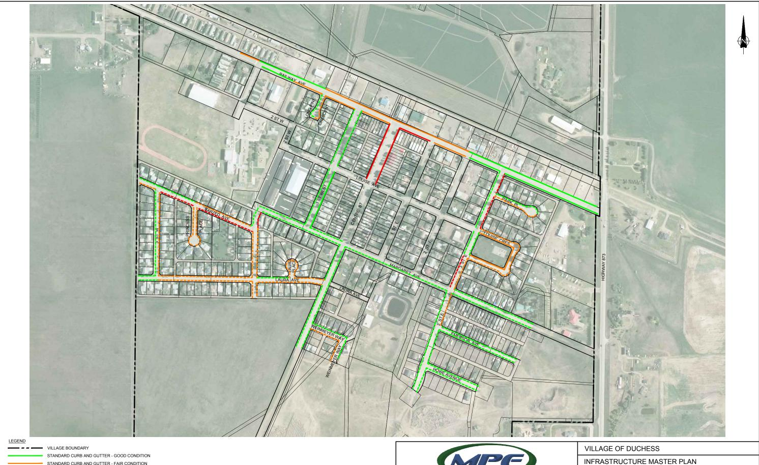
STANDARD CURB AND GUTTER - FAIR CONDITION STANDARD CURB AND GUTTER - POOR CONDITION ROLLED CURB AND GUTTER - GOOD CONDITION ROLLED CURB AND GUTTER - FAIR CONDITION ROLLED CURB AND GUTTER - POOR CONDITION
